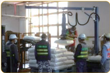
▲ Implementation of vacuum lifting equipment
