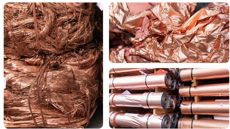
▲ Using 100% recycled wire / cable and factory-recycled Z-grade materials / copper trim scrap as raw materials for copper melting maximizes the use of recyclable resources, improves product efficiency, exceeds customer expectations, and moves toward net-zero emissions.
